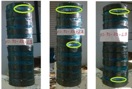
Fig. 3: Failure mode of HS-30-20 specimens
