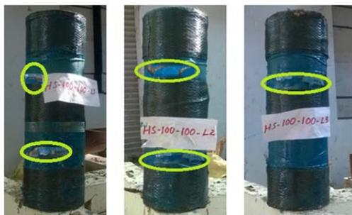
Fig. 5: Failure mode of HS-100-100 specimens
