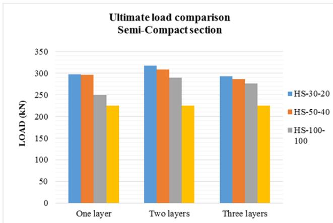
**Fig. 6: Ultimate load Comparison**
