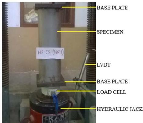
Fig. 1: Experimental Setup
