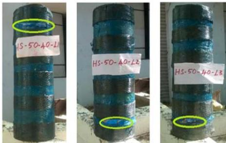
Fig. 4: Failure mode of HS-50-40 specimens
